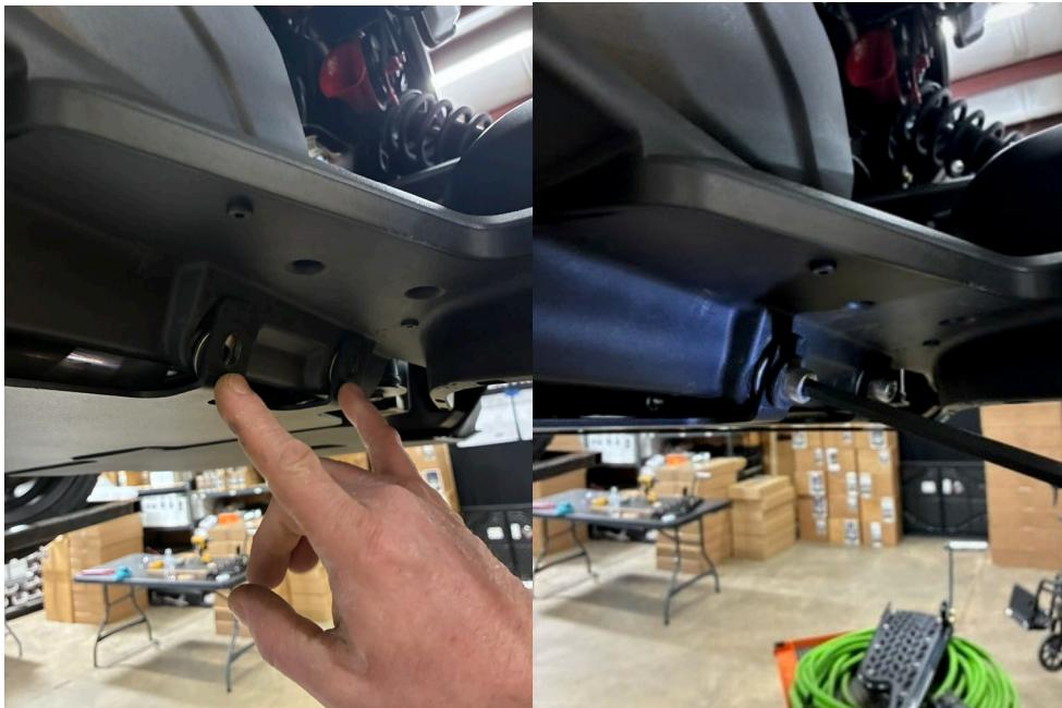
3.- Then take the floorboard such as the right side shown below and located the rear of the board where the OEM footpeg was located. Take the mount and now reattached the mount using the same bolts. Secure but do not fully tighten. Then secure the front with the two bolts used to hold on the plastic diverter. Use the supplied washers between the floorboard mount and the slot of the diverter. This acts as a spacer. Snug those bolts down at this point. You will need to make sure
