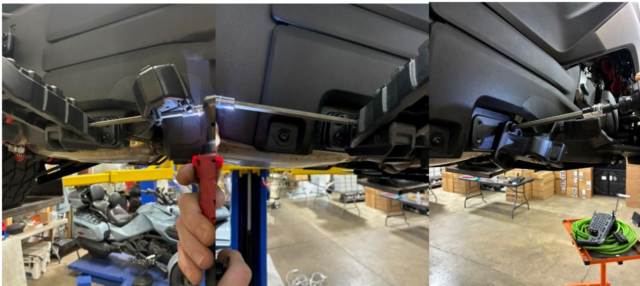
2.- Next use an 8MM Allen wrench and remove the two main bolts that secure the plastic diverter as shown below. Do this again on both sides.
