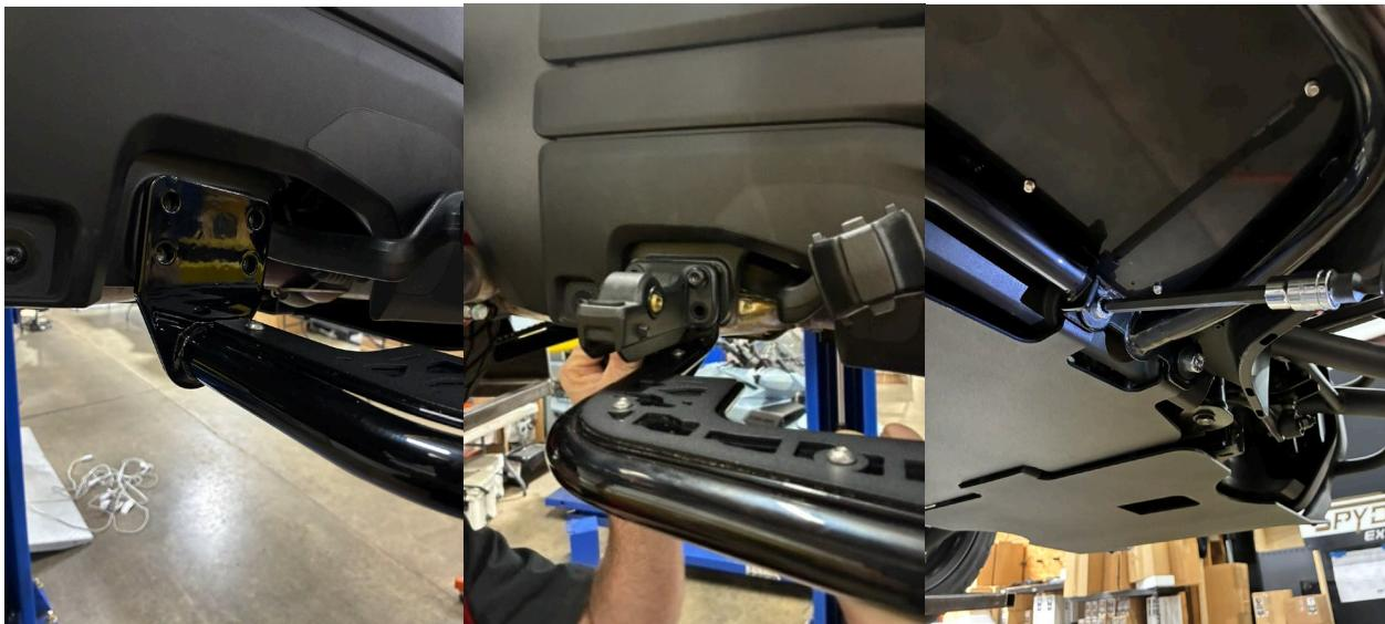
4.- Once all bolts are installed tighten up front and rear bolts evenly. Once the floorboard is secure then you can reassemble the footrest on the footrest mount.
