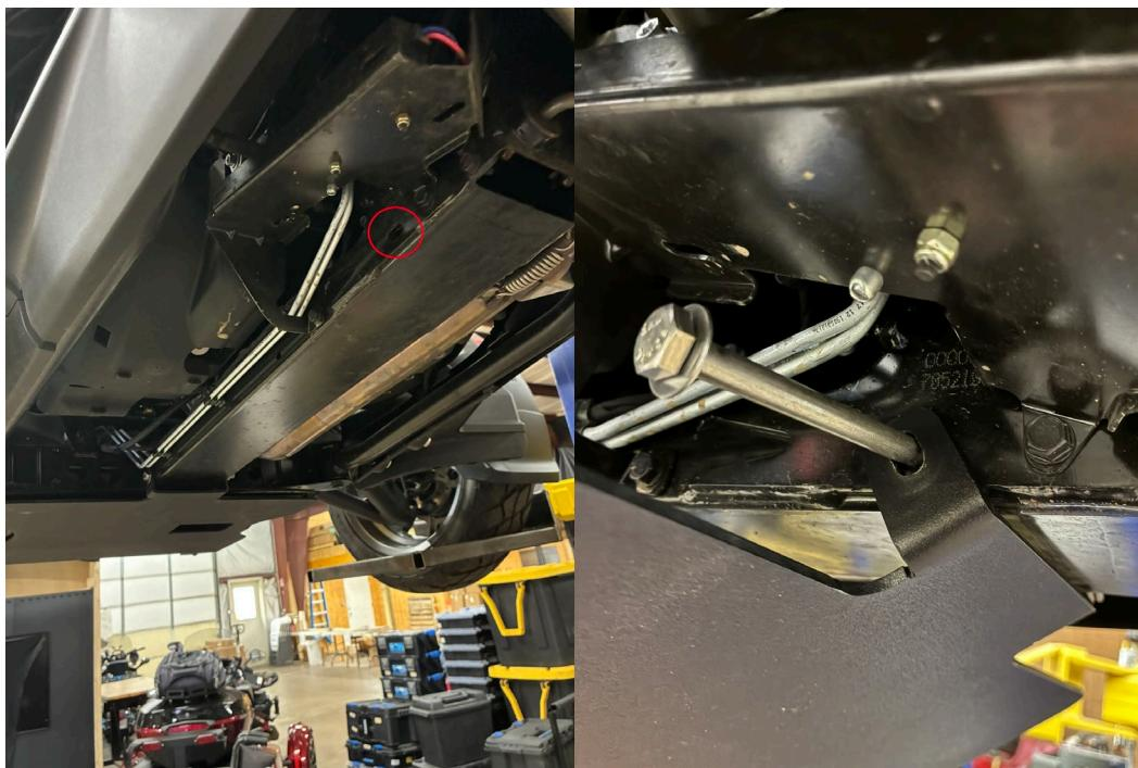
2.- Once the skid plate is in position take the 8mm Allen wrench and remove the two socket head bolts that secure the plastic deflector on each side. Next take the OEM bolts you just removed and take the supplied washer spacer and place the bolts through the skid plate as shown below. The washer spacer goes on the inside of the skid plate. These plastic deflectors will come off at this point and can be set aside.
