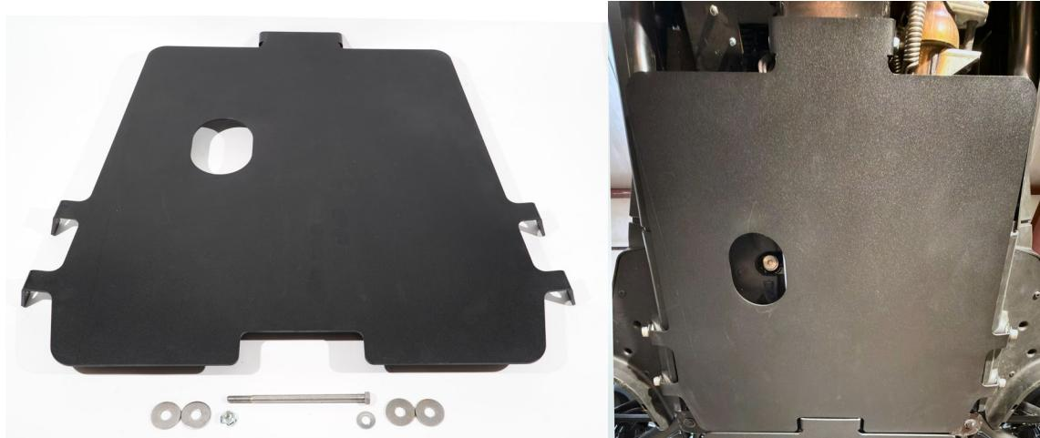
1.- To install the Rear Skid Plate, locate the hole circled in red on the lower photo. Take the supplied 5/16" bolt with the supplied washer and lift the skid plate rear U-Shaped mount and place over the frame as shown below. Run the bolt and washer through the plate and place the flanged head nut on the bolt and tighten light to allow the plate to hang from the frame.
