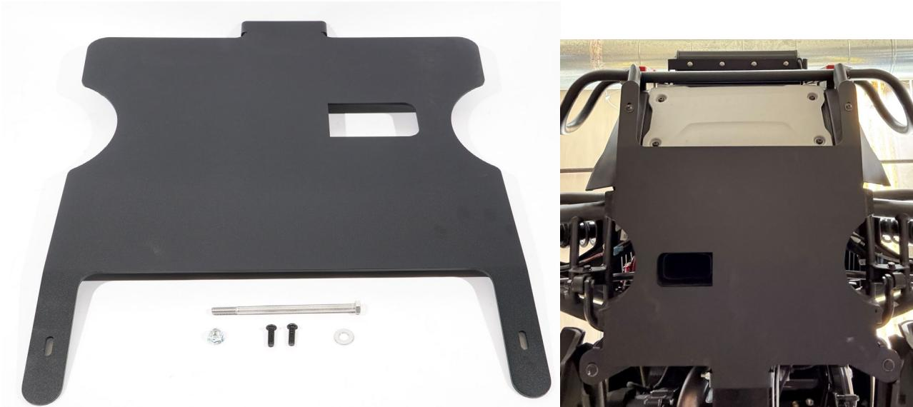
**1.- To install the front lower skid plate you will need two 1/2 wrenches & a 5/32 Allen Wrench. Locate the lower frame hole shown below that will secure the back of the skid plate. To simply install the skid plate, raise the skid plate into position as shown below . You will see that the skid plate back has two tabs that rest on either side of the main frame. Align the holes**
