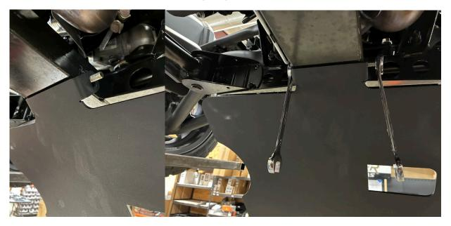
3.- Tile the skid plate upwards and take the suppled black button head screws and washers, using the 5/32 Allen wrench and secure the front skid plate tabs to the underside of the grille guard as shown. Do this for both sides.
