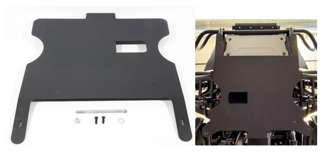
1.- To install the front lower skid plate you will need two ½ wrenches & a 5/32 Allen Wernch. Locate the lower frame hole shown below that will secure the back of the skid plate. To simply install the skid plate, raise the skid plate into position as shown below. You will see that the skid plate back has two tabs that rest on either side of the main frame. Align the holes
