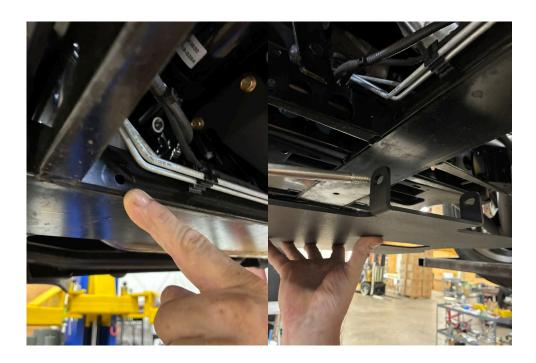
2.- Once the skid plate is in position take the suppled bolt with washer on head end of bolt and run the bolt through the skid plate as shown. Take the flange head nut on the opposite end and the two ½ wrench and tighten the bolt slightly at this point. This will allow the skid plate to hang down while you secure It to the front of the grille guard.
