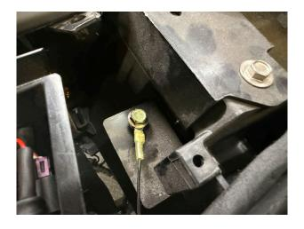
12.- Take the supplied two wire ties and bundle up the wiring harness to the existing harness and then the rest at the end together as shown below tucked away. If the new male connector is difficult to install over the female socket take a knife and make the guide slot in red below on the female abut 1 1/6" wider. This will allow a better alignment of the guide slot and the tab hanging down on the inside of the male housing to align the two connectors.
