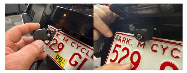
10.- Run the wiring harness form the camera to the connector location. Then take the supplied connector cable and plug the came into the red plug making sure to align the arrows and then connect the main connector as shown below. Notice the connection to properly fit the plug. Push in to lock in place.
