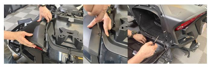
15.- Once all screws are back in position, take the passenger seat, plug it in and reinstall the seat either before or after installing the trunk.
