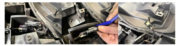
7.-Next take the 7/32 socket and unscrew the single bolt that holds the rear panel in place. Once removed take your hand as shown below and pull back on the rear light cover. Open it up about 4".
