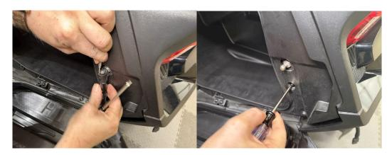
5.-Then use some screwdriver our plastic device and pull the side panel lose. Just pull lose so the top back corner is exposed.
