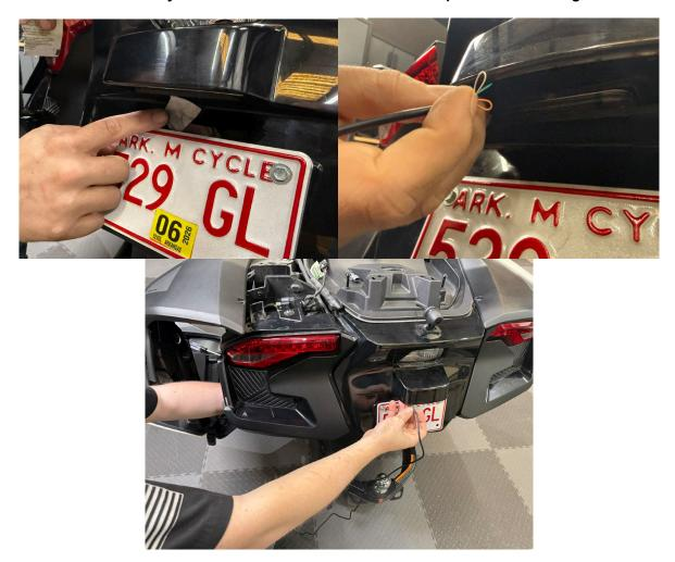
9.-To make sure the camera direction is correct the camera bracket as shown below should be able to tilt downward. Locate the camera center on your license plate as shown and stick the camera firmly in place. You can then tilt the camera up or down for best viewing.
