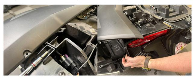
8.-Next take the supplied alcohol pad and clean the surface center above the license plate. This is where the camera will mount. Next take the camera wire and run it between the plastic cover and the license plate light fixture. Use your left hand to reach back behind and pull the wire through.
