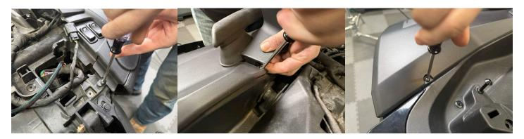
4.-Next with a small screwdriver unclip the gas spring. And lay down on the saddle bag door. Then with the T-20 wrench remove all side panel screws around the saddle bag face frame.
