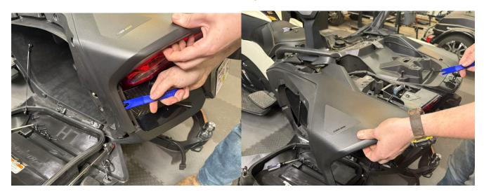
6.-Locate the backup camera main plug. It has a false end in grey as shown below. Then using a screwdriver our plastic pushpin puller, pry apart the two connectors by lifting the tab as shown below to separate the plugs.
