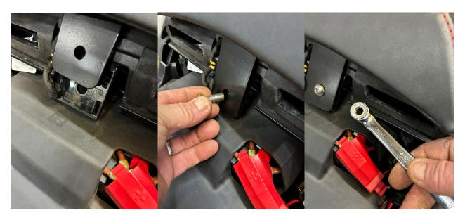
3.-Tighten down the bolt and then reinstall the driver's backrest. Next reinstall the driver's seat. Take a 3/6" Allen wrench and adjust the tilt angle bolt of the backrest as shown to fit your back for comfort. Turning the bolt clockwise tilts the backrest forward. Your Drivers backrest is now installed!
