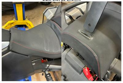
2.- Next slide the backrest bar down to the mount shown, then take the supplied bolt and flange nut and place the bolt through the hole and place the nut on the back using the boxed wrench to help locate and hold the nut while assembling. Using the 7/32 Aleen wrench, tighten down the bolt which secures the backrest mount.
