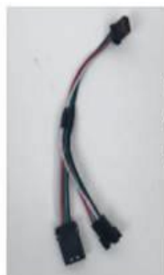
WIRE A TAIL LIGHT Y-WIRE
