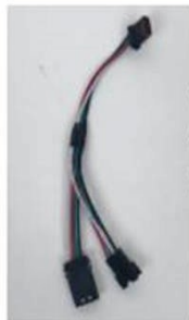
WIRE A TAIL LIGHT Y-WIRE
