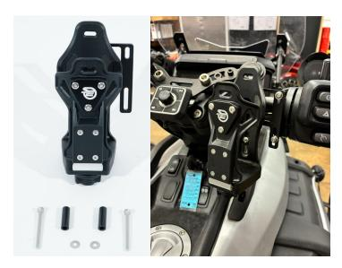
1.- First with a 3mm Allen wrench remove these two OEM screws at the back of the handlebar cuff as shown below. Next take the cup holder, spacers, washer and bolt and place a space top and bottom between the cupholder bracket and the cuff. Take the washer and socket head bolt provide and screw the top and bottom bolts in as shown below and tighten evenly. If you want the cup holder on the opposite side, simply remove the bracket from the cup holder and flip it over and reassemble it.
