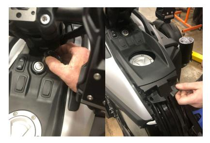
4.- Next take the supplied switch and place it into the switch housing as shown below then seat the switch.
