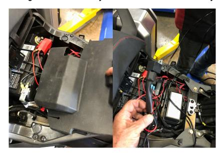
5.- Take the white plug from the switch and plug it into the white plug form the relay harness. Take the two leads out to the Light Pods and run them up the center area then secure under the oem tab holding wires secure.
