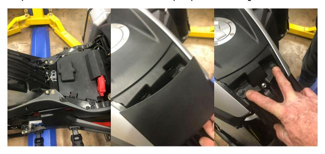
3.-First twist the plastic nut around the ignition key as shown below. Lift-up the plastic housing and locate the lower right blank switch cap and remove it.
