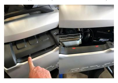
7.-The run the remaining wire from the switch with the Y-Adapter attached and plug it into the OEM accessory wire as shown below. This wire is tucked up in the upper left corner in the side location. This powers the switch that turns the relay on or off.
