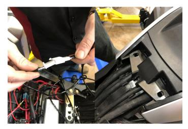
6.- On each side remove the upper access panels as shown below. This photo is the left side.
