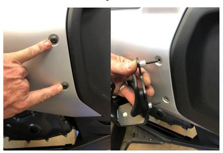
2.-Once mounted, you have 3 positions for the cup holder. Stright up or rotate it towards the rider in 2 other positions, shown below. You can adjust the cup holder using a 3mm Allen Wrench.
