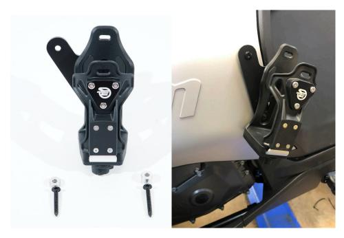
1.- First with a t-25 Torx wrench remove these two OEM screws. Next take the cupholder if mounted on the drivers left side as shown here and take the longer suppled screw and spacer on top and the smaller screw and spacer on bottom and place the cup holder as shown below. The lower shorter screw mounts through the cup holder & lower bracket hole first then which allows the cup holder to rotate. The upper longer screw and spacer mounts the mounting bracket alone.
