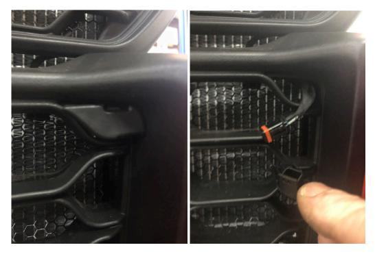
5.- Using a T-30 Torx wrench, remove the top two bolts as shown below each side and only loosen the lower two. Once the front rails are loose, install the supplied plastic spacers as shown. They are designed to fit the rail. Do this for each side.
