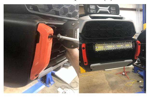
Make sure the top switch cover is reinstalled as it was removed and install the driver seat. Your new Canyon Light Bar is now installed.
