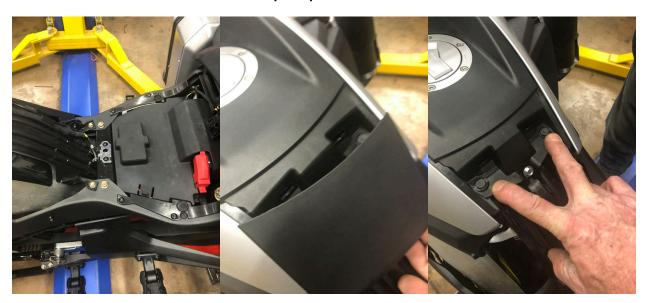
2.- Once the rear panel below the seat is removed remove the upper panel surrounding the ignition switch and switches. First twist of the plastic nut Around the ignition key as shown below. Lift up the plastic housing and locate the upper right plastic switch cover and remove it.
