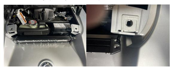
7.-Once the Light Bar is in place, return to where the plug is located and plug the light bar into the remaining socket. Then turn on the key and test the switch as the light should come on. If so, you have completed the installation. Take the wiring plug below and tuck it back up behind the fender where the OEM original socket is located. Make sure the top switch cover is reinstalled as it was removed and install the driver seat. Your new Canyon Light Bar is now installed.
