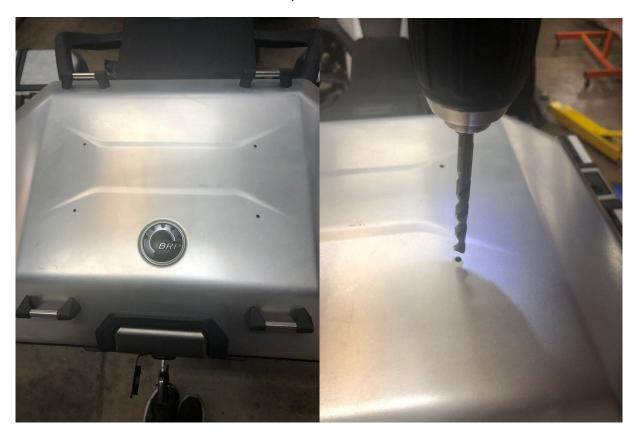
3.- Take the rack and flip it over. Take the 4 supplied bolts and rubber spacers and place a bolt through the hole and rubber spacer as shown below. Do this for all 4 spacers. Next take the rack and place it on the trunk. Raise the trunk and place a washer and locknut on each bolt. Take a 4mm Allen wrench and a 7/16" socket and tighten down each bolt evenly to where you start to see the rubber spacer compress. That insures a watertight seal. Your new rear trunk rack is installed.
