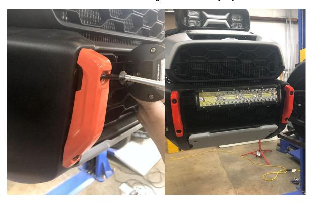
Make sure the top switch over is reinstalled as it was removed and install the driver seat. Your new Canyon Light Bar is now installed.
