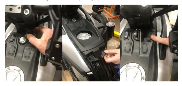
3.- Locate the switch wire harness that was below the plastic switch cover you just removed.
