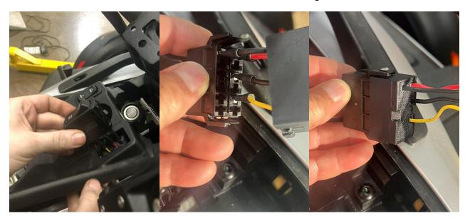
4.- Reinstall the cover in reverse of how it was removed and place the plastic nut around the ignition key area. You can test it as shown as the Amber light will glow.
