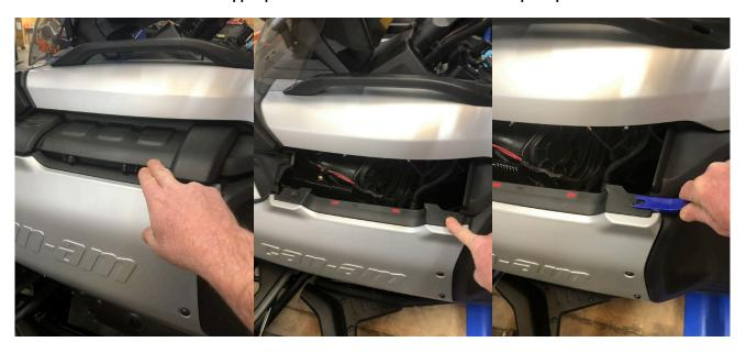
3.- With a T-30 driver remove the upper screw as shown. Then remove the upper panel. Pull the upper right panel outward to unclip and then slide rearwards to remove.
