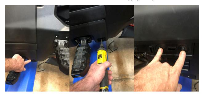
2.-Next remove the upper panel as shown below. Then remove the push pin as shown.
