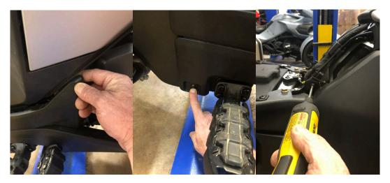
5.- Once the upper panel is removed, then locate the factory horn. Remove the horn by removing the bolt as shown below. Then take the new horn assembly and secure it as shown with the new nut and bolt. The washer and locknut go on the back side. Tighten up the bolt.
