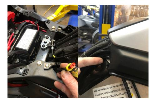
7.-Then take the existing factory horn wires and on each side of the positive and negative plug clip off the small tabs on each side. This will allow those wires to slide into the new horn harness plugs.
