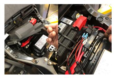
2.-Next remove the cover as shown below. Push in on the two tabs of the cover and then remove.
