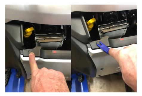
4.-Next remove the lower panel by pulling this panel at this location. Then remove this screw below. Then remove the upper panel but pulling the upper right side down to unclip then forward to release.
