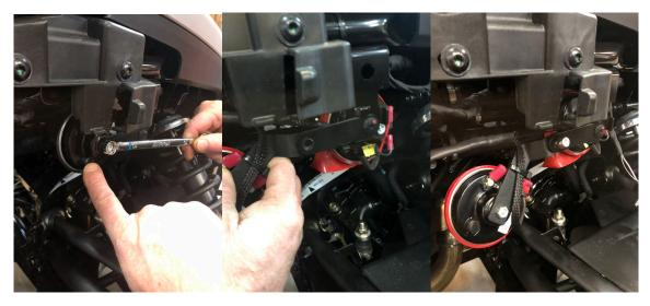
6.- Once the horn unit is installed take the wiring harness ends from the battery location and run those wires along the frame and under the metal panel and out as shown below. Then run the wires behind the panel as shown then to the horn location.
