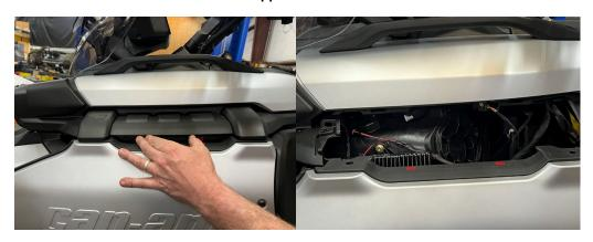
4.-Next remove the two push pins one on each side as shown below. Then locate the front panel below and remove the two metal keepers and then remove this panel.
