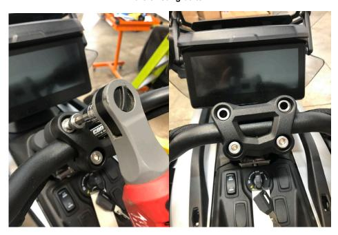
2.-With the supplied new socket head bolts and aluminum spacers, place a spacer in each hole on the steering wheel. Be gentle in making sure they stay in position. Take the two new socket head bolts and washers using 8mm Allen wrench, apply medium strength Loctite (Blue Color) to lower ½ of the threads to secure once you tighten down firmly to manufactures specifications.
