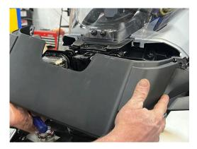
6.- Look inside on as shown and located the factory accessory plug. Once located direct the plug wire through the hole in the plastic as shown.
