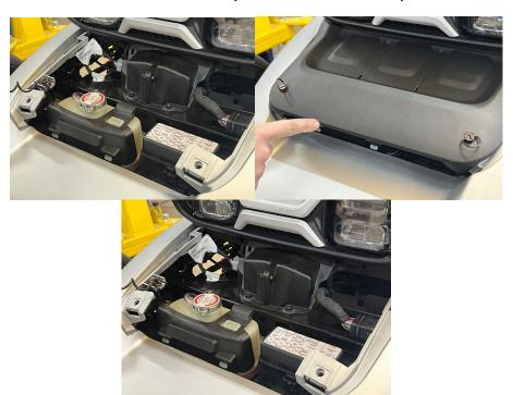
5.- Once the panel is removed then grab the LED headlight case and remove this.
