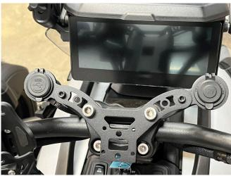
1.- Remove the top two socket head bolts from the center steering column using a 7mm Allen wrench or socket. There is a total of 4 bolts remove only the top two bolts. When removing them please keep the two washers from the existing bolts.
