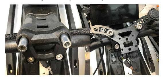
3.-Your Canyon CAN-1U12ADJ, 12-volt power station is pre-wired at the 12-volt sockets. You will need to connect to the accessory plug on the LEFT side aux power supply plug. First remove the panels as shown below. Squeeze in on these two tabs to remove this access panel. Remove the panel. Do the same for the panel on the opposite side.
