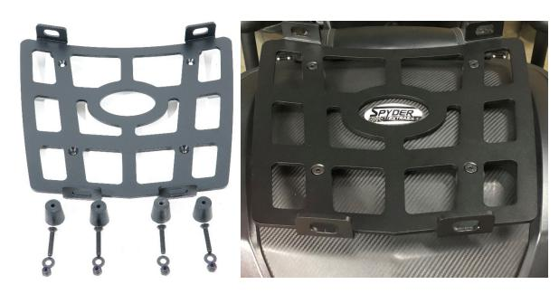
1.- First raise the lid of the Trunk. On the underside you will see two ridge lines from side to side as shown below. Take the supplied template and located it as shown below in the 4 positions one at a time. The template lines up with the ridge line then located to each side as shown. Once located, use the hole in the template using a ¼" drill bit and drill the 4 holes required. Then use a 17/64" bit to make the holes larger for easier access of bolts.
