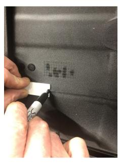
2.-Once all 4 holes are drilled as shown below. Then take the rack and supplied rubber spacers and run each bolt through the rack into the spacers as shown. Flip the rack over to install the tapered rubber spacers with narrow side to the rack. Once all spacers are in place turn the rack back over and install the rack into the trunk. Then take the washers and lock nuts and install each on each bolt and tighten down evenly to where the bolts come through the lock nut at least 2 threads.
