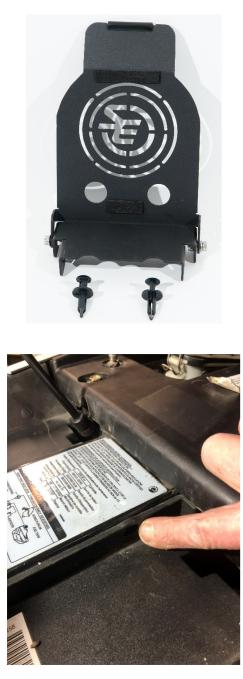
2.- Then take the assembled lift kit and place the main lower mount over the frame so the lower bracket holes line up with the holes above in the frame.
