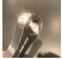
Take the install Nylon Insert and place it through the link top bearing. Place one spacer each side and you will see that the spacers once added fit flush with the nylon insert from side to side. This will hold
