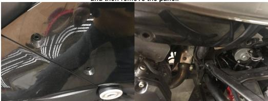
3.- Remove the rear existing Factory Footrest4.-Insert the black Nylon MD spacer in the Rear Footrest cradle.
