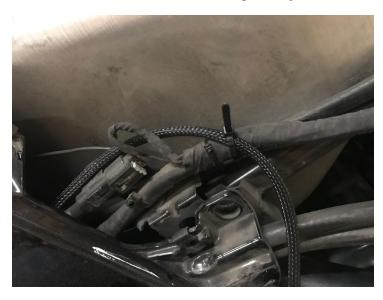
8.- Remove the left side Footrest as you did the right side and repeat the above process. This left side LED wire is shorter, and it can be run along the inside of the panels to the upper left area access panel using wire ties as you did on the right side. Connect the Red LED wire to the other open Positive Lever Connector and the Black the same to the Negative Lever Connector
