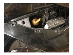
2.- Remove the two bolts each end of the right-side Panel and then remove the panel.
