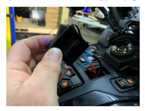
11.- If your light bar wires get unplugged from the switch, the light bar wires plug into the ground wire on the switch / blue spade and the open terminal as shown below on the lower left next to red positive wire is where the positive wire from the light bar plugs in shown in the photo.
