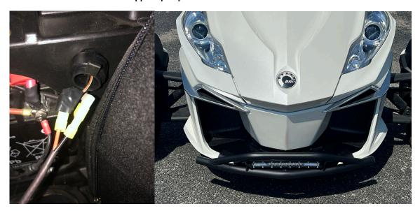
6.- Once the switch wires, suppled power & LED Light bar wires are run to this one location, plug all wires into the switch based on how they are labeled. Besure to connect red to red / black to black. Take the supplied wire ties and tie up the wires as shown. Now you need to test the light bar. Turn on the Key Switch and go through the motions of powering up the Spyder. Once done push the switch to make sure the light is working.
