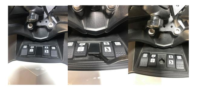
2.- Take the suppled new switch cover and switch and run the wires from the switch through the plate as shown below.
