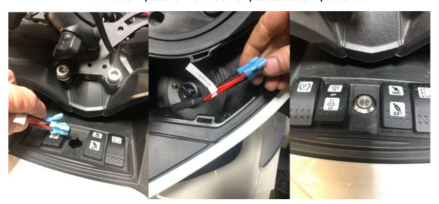
4.- Remove the right-side access panel shown below. If you have never removed this panel, it may be snug so apply pressure to remove. Using a long wire or wire tire as a guide run the switch wire down to come out of the panel area as shown below. This is where you will connect the power cable from the accessory location next to the battery and the light bar wire. You will connect all wires to switch here last.
