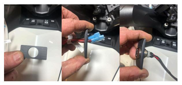
3.- Take the switch and remove the adhesive tap from the back of the switch face plate. Be sure to clean the area around the hole where the switch plate will set. Remove the right speaker grill and run the switch wires down through the hole and retrieve them in the speak area as shown below. Remove the tape backing, Insert the switch in the hole and press down on the switch plate to secure in position.
