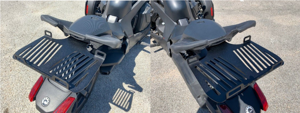
Rack shown in the #2, back slot position allowing the rack closer to passenger.
