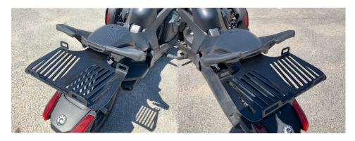
Rack shown in the #2, back slot position allowing the rack closer to passenger.
