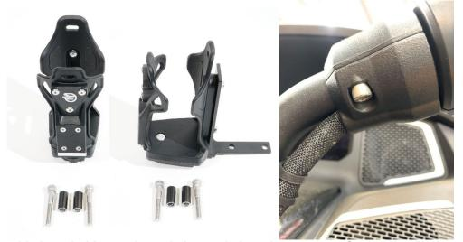
Then take the preassembled cup holder as shown below and place the new 6mm Socket Head bolts w/ Spacer between the bracket and the factory module mount.
