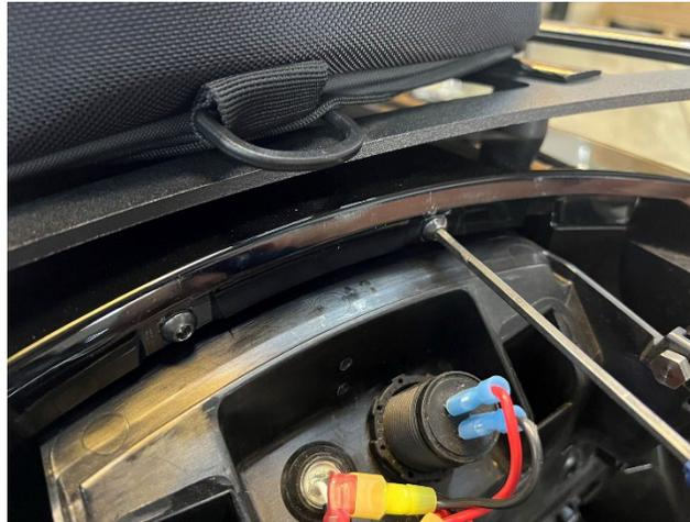
**5.- Next take the upper lift kit mount and insert it from the trunk area so the mount tabs align with the two holes from the screws you just removed. Then take the 2 new supplied 6mm black screws and secure the mount to the trunk housing.**
