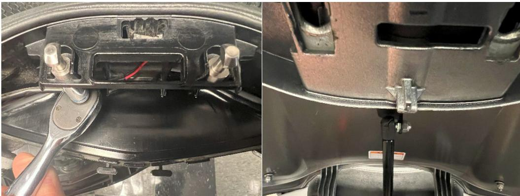
Your NEW Lift Trunk Lift kit is now installed. You will enjoy the ease of opening the trunk as it lifts automatically once the latch of the trunk is pushed and you start to lift the lid. Too, the lift kit will lift an extra small luggage bag etc. you might have on the optional trunk rack.
