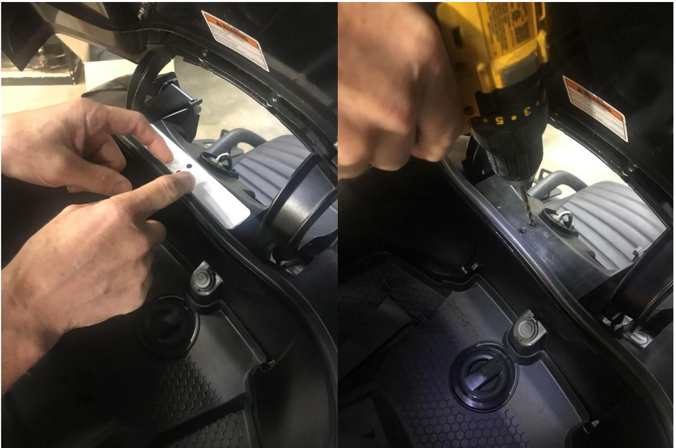
**Option 2 Upper Mounting Position USB Lower Placement. Drill two holes.**
