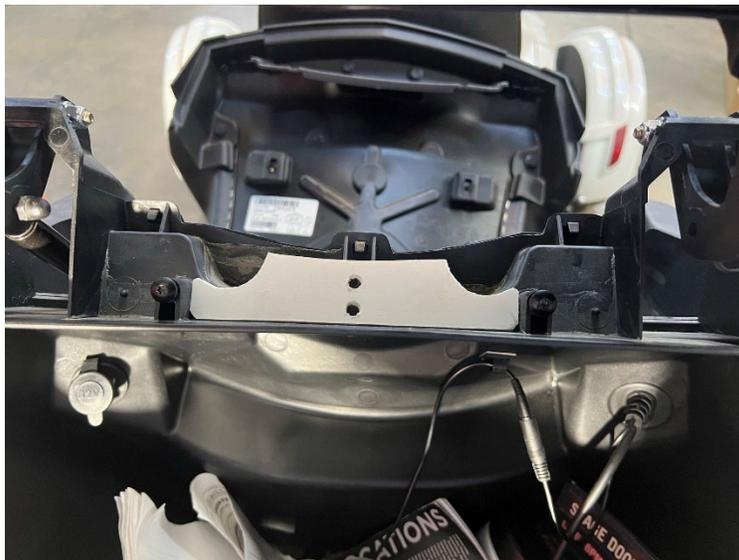
**4.- Once the two holes are drilled, take the lower mount and the two supplied black T-20 screws and locknuts, and secure it to the trunk housing as shown. Use a 10mm wrench on the two lower locknuts to tighten them down. Finally take the gas spring with the larger receiver section of the spring at top, snap the spring on the upper ball and the same for the lower ball. Your Trunk lift kit is now installed.**
