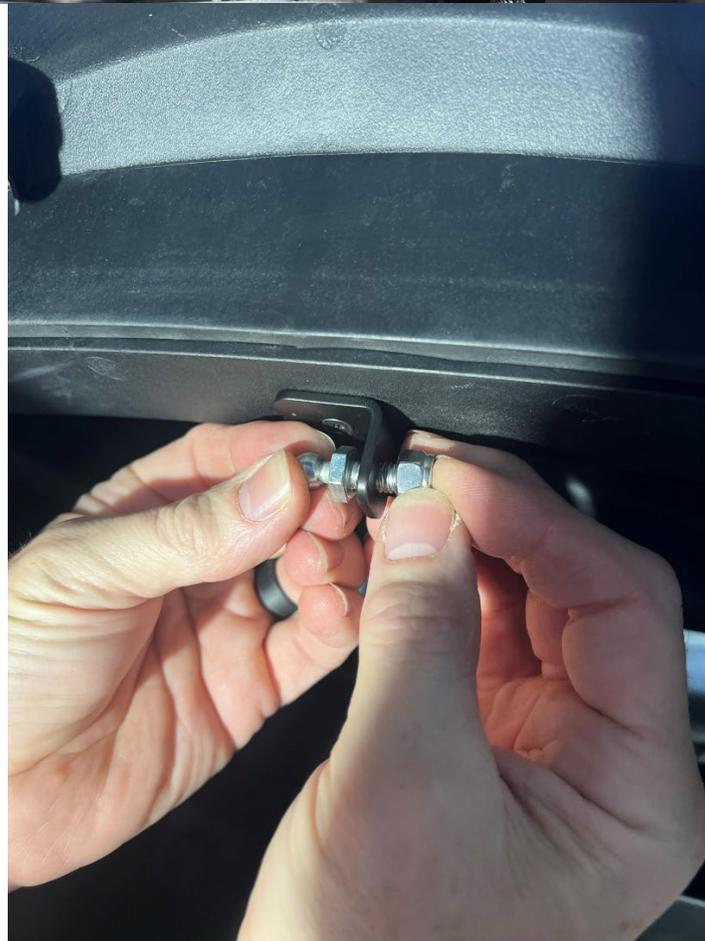
**2.- Next remove the passenger back rest by removing the 3, T-25 screws using the T-25 Torx wrench in the trunk. Then using the T-20 Torx wrench loosen the T-20 screws on the back seat panel as shown. Once those screws are loosened then remove the rear passenger backrest.**
