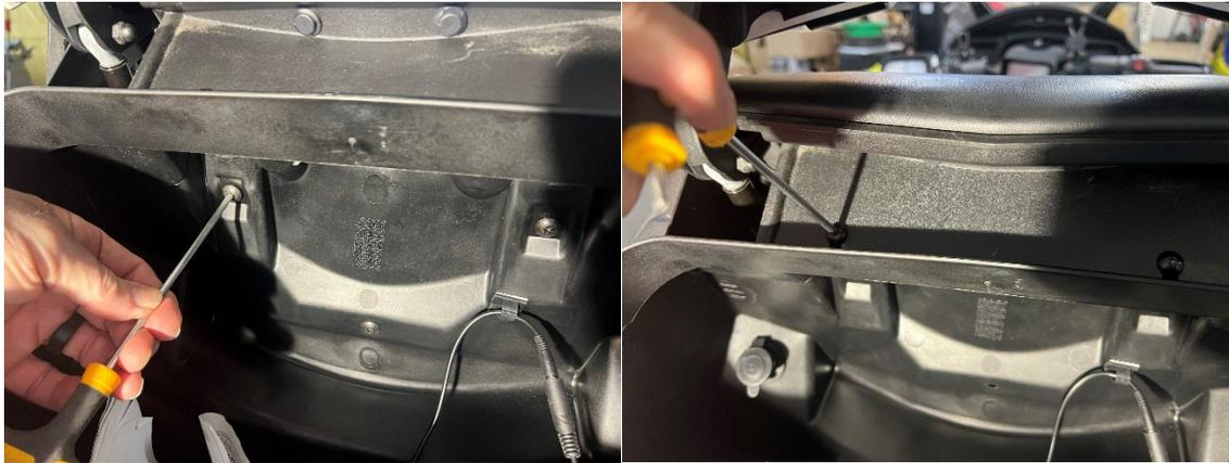
**3.-Take the supplied template and place it in the space as shown below. It's designed to align perfectly. Then take a 7/32 drill bit and drill two holes through the template for the lower bracket mount.**
