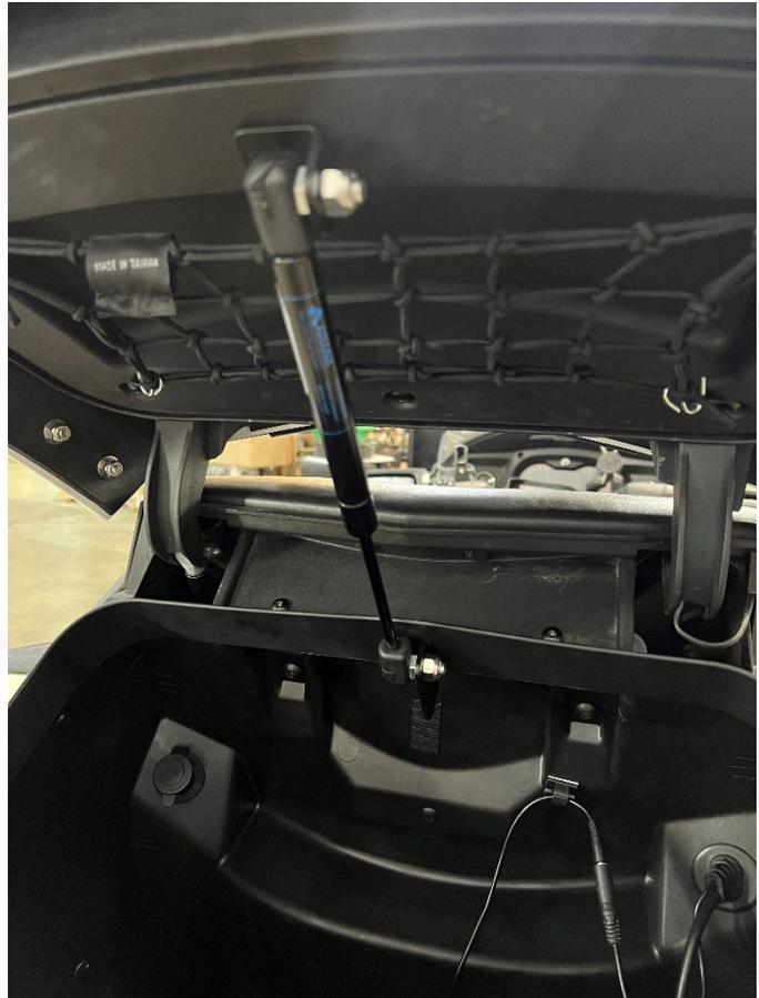
1.- First remove the center screw using a T-20 Torx wrench. Next take the upper mounting bracket. Remove the 3M tape back. Place the bracket in the center screw hole location and press the back of the bracket to the trunk lid to hold it in place. Next take the supplied new T-20 Screw that will recess into the bracket and tighten down. Then take the supplied ball mount and using 1/2" wrenches secure the ball to the mount as shown below.
