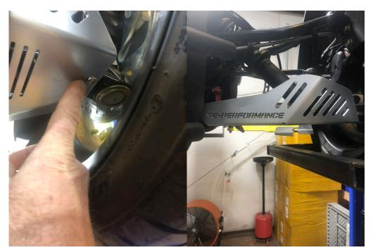
2.- Next remove on the left side only the Ryker the upper cover panel by removing the pushing pins as shown below in these locations. Once all push pins are removed, remove that panel to access the factory accessory plug.
