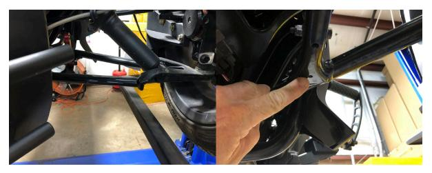
2.- Locate the correct shield per side and place under the A-Arm. Then take the 6mm screw and 4mm Allen Wrench and secure the shield to the arm as shown below. Do not tighten the screw at this point. Just enough to secure the shield. Then take the two 5mm screw & the 3 mm Allen Wrench and secure the rear of the shield to the arm placing the screws through the shield and then add the washer and locknut per screw. Now tighten down all screws.
