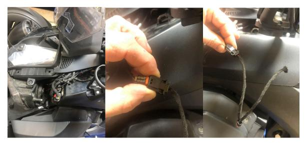
5.- Once the Y-Adapter is plugged in to the accessory plug, you are now ready to run the wires from the LED Light strips on each shield to this accessory plug. This setup is all Plug & Play.
