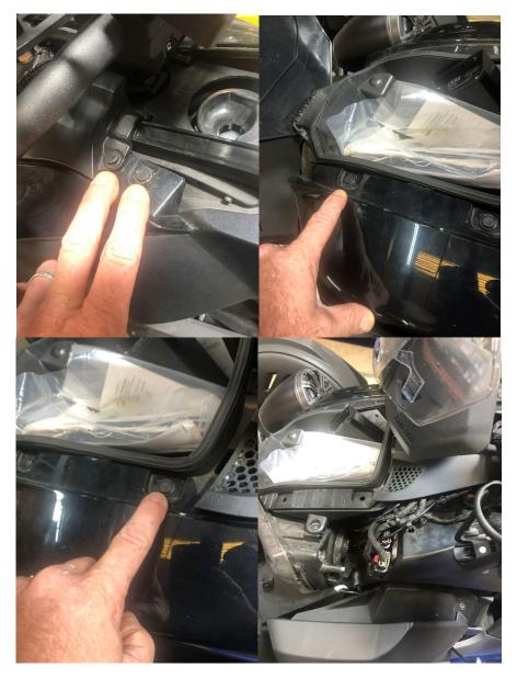
4.- Take the factory accessory plug and connect it to the supplied Y-Adapter supplied to allow connection of the LED Lights in the A-Arm shields.
