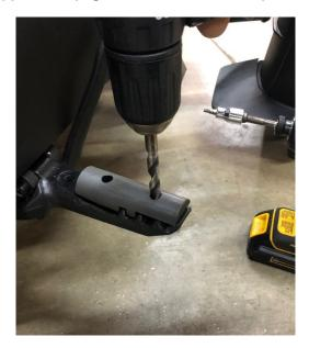
2.- Once both holes are drilled take the Floorboard support mount as shown below and locate the mount over the spacer on the foot peg. Take the two 5/16" Socket Head Bolts and place the floorboard main support over the footrest and take the mount lock plate flat side up and mount it from the bottom as shown below. Screw the bolts down evenly through the mount then the footrest into the mount lock plate. Tighten down evenly through the lock plate then add the safety locknuts as shown below.
