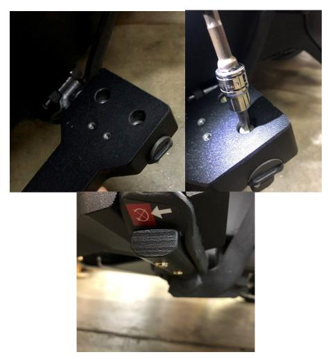
3.- Before permanently securing the floorboards to their mounts adjust the floorboards to your riding position. This needs to be done before the floorboards are secured to the mounts. If you have more than one rider of the Ryker, the boards "only" will need to be removed each time by removing the two center screws to reset the peg mount locations for each rider. Then install the boards.
