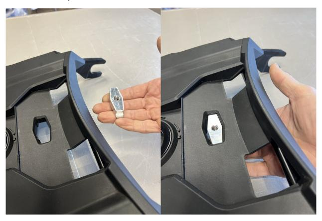
2.- Next take the base mount plate and secure it to the LinQ mount. The plate secures to the LinQ with the two hooks that loop under the bar in the LinQ mount. Once in place take the Socket head bolt and washer and secure the base plate to the LinQ mount. Tighten down the bolt.
