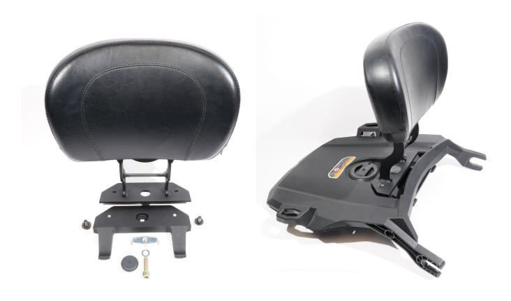
1.- You must have the BRP LinQ mounting rack for the 2020+ RT base models. Next take the Aluminum lower lock plate as shown below and locate it underneath the slot as shown.
