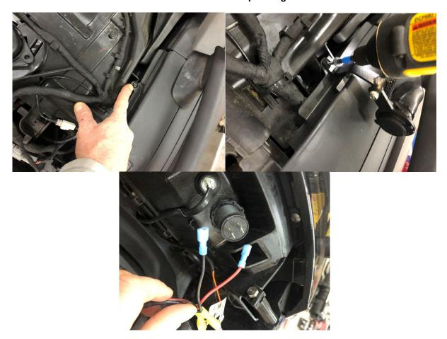
3.- On the Spyder 2020+RT base model with no trunk you will use the wire harness adapter plug shown below for this kit. Once you remove the passenger seat as discussed above, locate the factory harness and plug the adapter into the OEM harness. Then take the positive and negative wires from plug and plug those into the yellow terminals making sure to match red to red / black to black.
