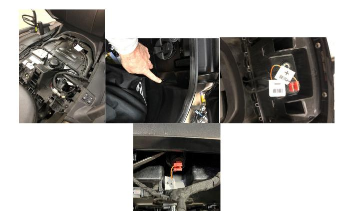
2.-Take the new USB mount and remove the factory screw as shown below. With the new screw provided place the new USB mount as shown below. The mount bracket has a cross bar that rest against the panel of the spyder as shown. Tighten down the screw.
