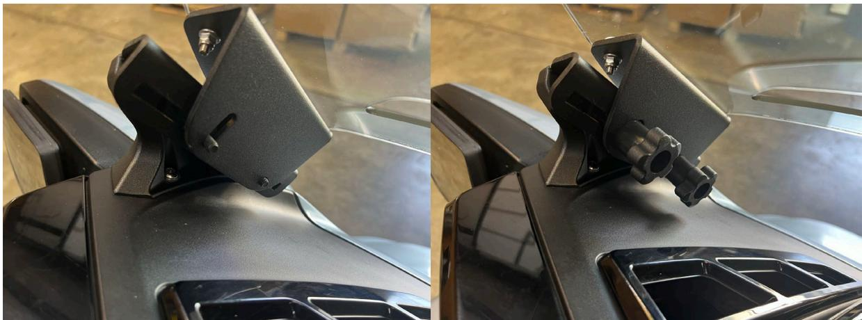
5.- Once the shield is installed then adjust it to how you want to ride. The shield will raise and lower as well as tilt in and outward. Experiment to see what best fits the way you ride and how much airflow you will want compared to stock settings. First time using the knobs the locknut will be tight when turning the knobs. Once tight in the position you like to adjust is much easier. Then add the black plastic cap covers for a finished look on the outside of the shield.
