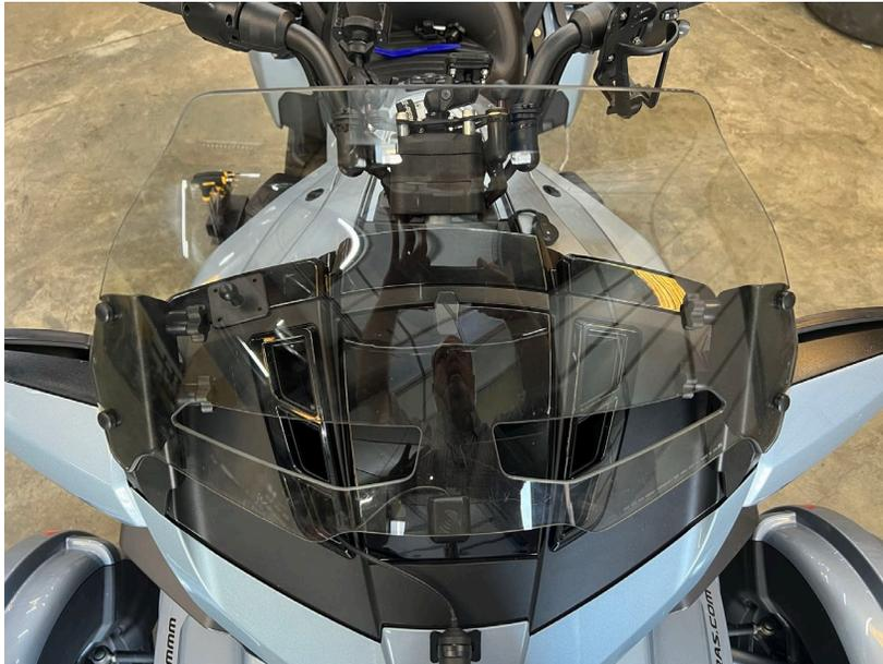
5.-If you install an aftermarket windshield such as the F4 Customs or other brand, use their supplied shield bolts to secure the shield to the mounts. Follow the manufacturer's instructions for installing their shield to the adjustable mounts.
