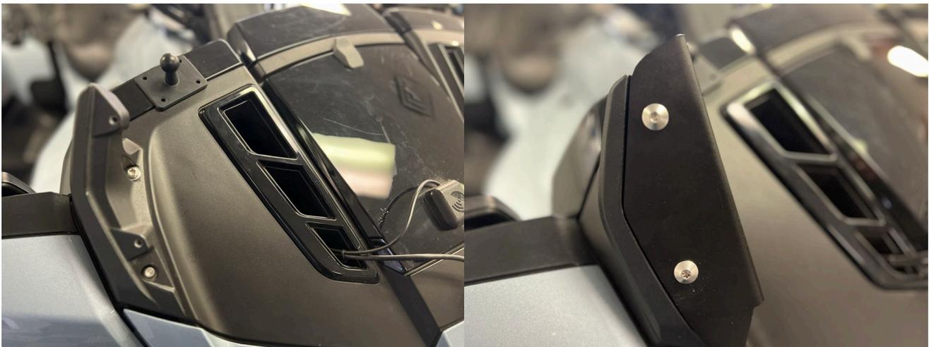
**2.- Add the lower carriage bolt through the main mount slot and through the lower hole on the shield mount as shown. Add the rubber supplied washers on each carriage bolt. The washers will help hold the bolt in place. Do the same for the Right side as shown below.**
