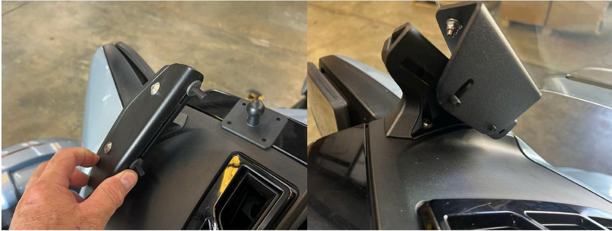
**3.- Simply take the OEM windshield with the newly supplied clear cap mount with the supplied shield 5mm bolt and place the left bracket and align it with the shield before tightening down the locknuts. Once the bracket is aligned with the shape of the shield tighten down the locknuts. Once the left shield mount is installed do the same for the right side. Use a 3mm Allen Wrench.**
