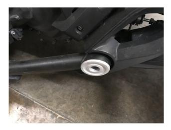
3.-Take the Floorboard and the two supplied 8mm button head bolts and small angled spacers and install the lower mount bolts and metal OEM existing lock plate on the back side as shown below.
