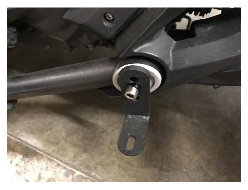
6.- The rear board hanger bolt, depending on where the front mount riding position is located as discussed, that bolt will use one of the rear holes for proper alignment as shown below. Once all bolts are located tighten all down.
