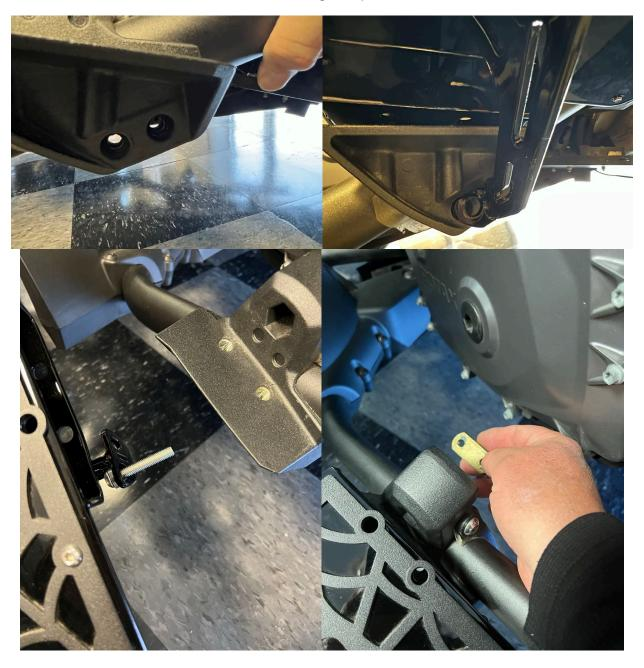
4.- Next install the two top 10mm bolts to secure the floorboard. Do not tighten at this point.
