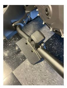
2.- Remove the rear frame support arm bolt.
