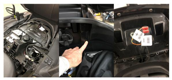
2.-Take the new USB mount and remove the factory screw as shown below. With the new screw provided place the new USB mount as shown below. The mount bracket has a cross bar that rest against the panel of the spyder as shown. Tighten down the screw.
