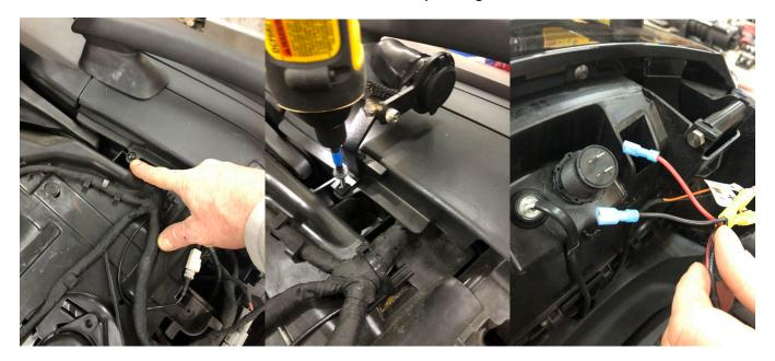
3.- On the Spyder 2020+RT base model with no trunk you will use the wire harness adapter plug shown below for this kit. Once you remove the passenger seat as discussed above, locate the factory harness and plug the adapter into the OEM harness. Then take the positive and negative wires from plug and plug those into the yellow terminals making sure to match red to red / black to black.
