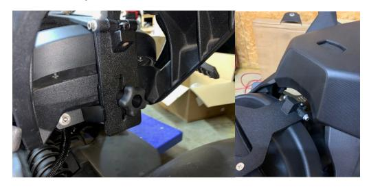
5.- If you install the Backrest and do not use the Max Mount / Passenger Seat, use additional Grade 8
