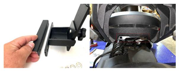
3.- Take the two 5/6" Socket head bolts with a washer on the outside of the lower mount bracket and one on the outside of the L-Bracket and apply the locknut and tighten down each side making sure to make the system level.
