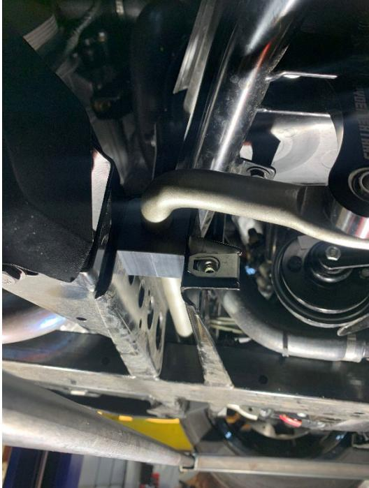
**Insert the new sway bar reverse of how you removed the existing. Be sure to take note of the location of the sway bar bushings. Using the supplied grease, grease the inside of the bushings then install the new bushings in the exact locations as the factory installed bushings. Insert the existing bolts and tighten down the nuts holding the bushings in place.**
