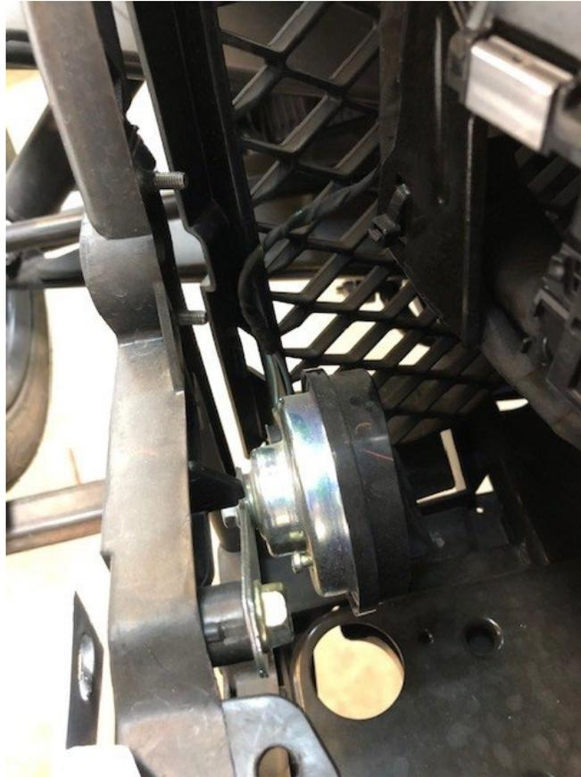
**4.- Take the new horn kit with the new bolt and spacer provided and locate the new kit in the same place as the factory. The dual horns will have both horns openings pointing down.**
