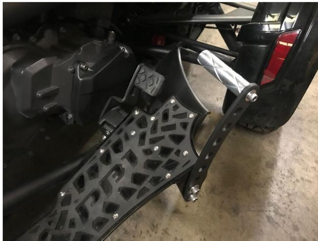
**7.- Next take the existing brake pedal pad off the brake pedal arm. Remove the two bolts from bottom side. Take the supplied spacer and new bolts and add the spacer between the brake pedal pad and the brake pedal mount. Secure using the two longer bolts. This allows your brake pedal to have additional room for your new floorboards.**
