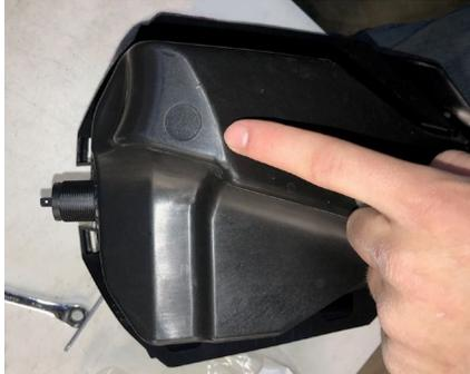
6.- Next take the wire and locate as shown in the pic below. The end result will be the wire connectors will be located under the front box as shown on the right photo below. Take the main harness with the positive and negative wires and run from this front box location down to the battery. Make sure the harness is free from moving parts and the steering arm. You can wire tie it up later.
