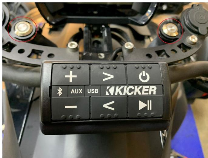
9.- Run both switch wires down through the steering column each side along with the factory wires. Run the switch wires to the front of the box area with the other cables and plug back into the flip connectors as before. Be sure Switch A & B plug back into the correct connectors. This is the main harness connectors that have only two flip levers each.
