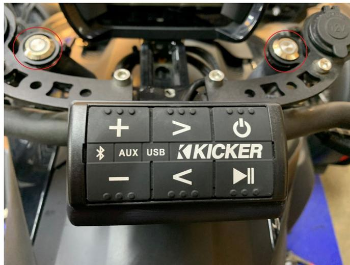
9.- Run both switch wires down through the steering column each side along with the factory wires. Run the switch wires to the front of the box area with the other cables and plug back into the flip connectors as before. Be sure Switch A & B plug back into the correct connectors. This is the main harness connectors that have only two flip levers each.
