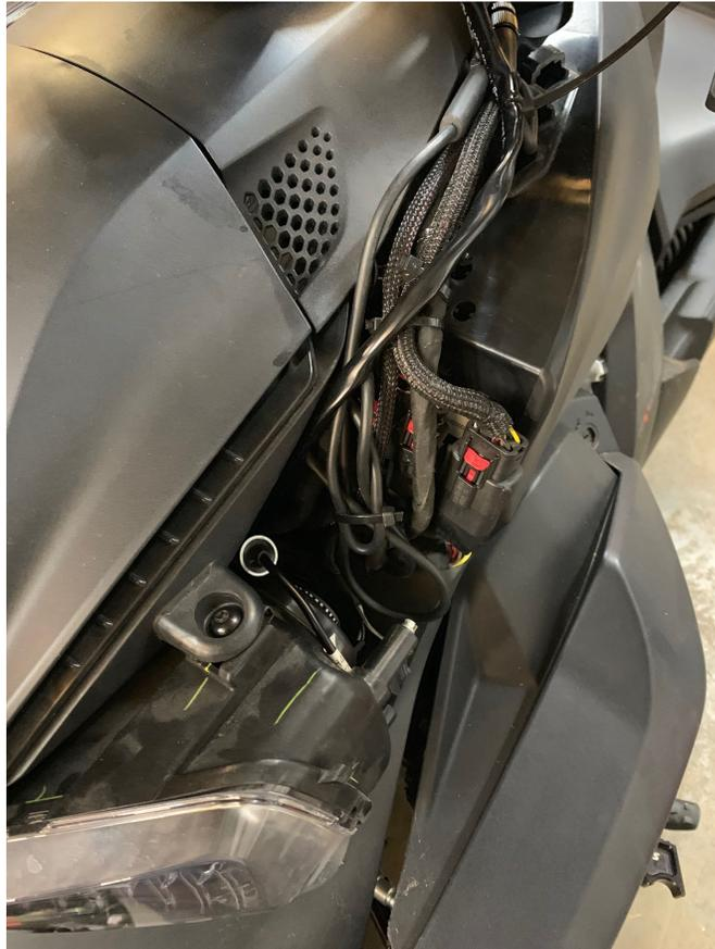
**Remove the Left side panel as shown by removing the push pins connectors**
