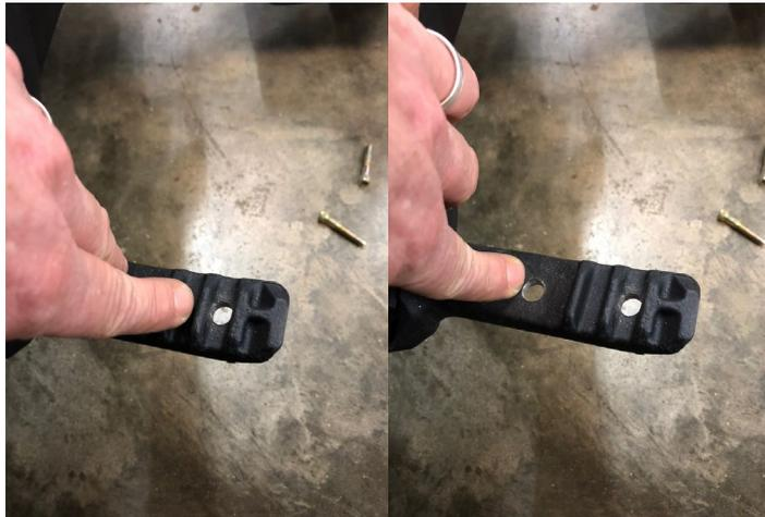
7.- Then install the main mount and floorboard as shown above. The lower lock plate on this version, make sure the lock plate flat portion is up against the bottom of the peg as shown below. Use Blue LocTite on bolts to lock plate
