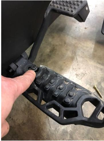
6.- Next drill a 5/16" hole shown below center of peg support as shown below on left photo below. Then take the floorboard mount main bracket lay over the mount drop a bolt in this hole for alignment and then drill another 5/16" hole as shown below on the right photo. Next drill out these two holes with an 11/32" drill bit to allow for adjustment when bolting together.
