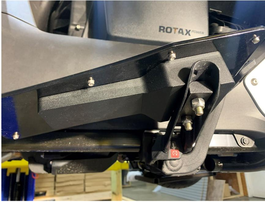
3.- Take the floorboard plate with the letter R facing outwards and the two button heads screws and screw the floorboard plate down. Do the same for the opposite side.
