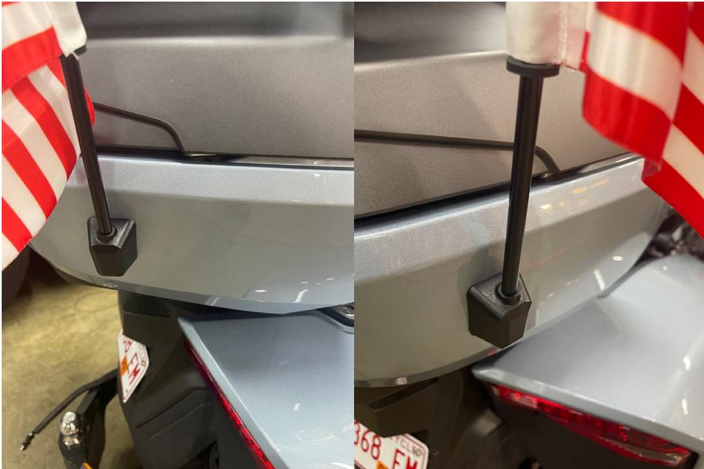
4.- Once the flag is located on the outside as shown above tighten down the inside bolt to secure the flag in place. The small flag holder 7/32 hole is for a stub that prevents the flag from moving once tightened down.
