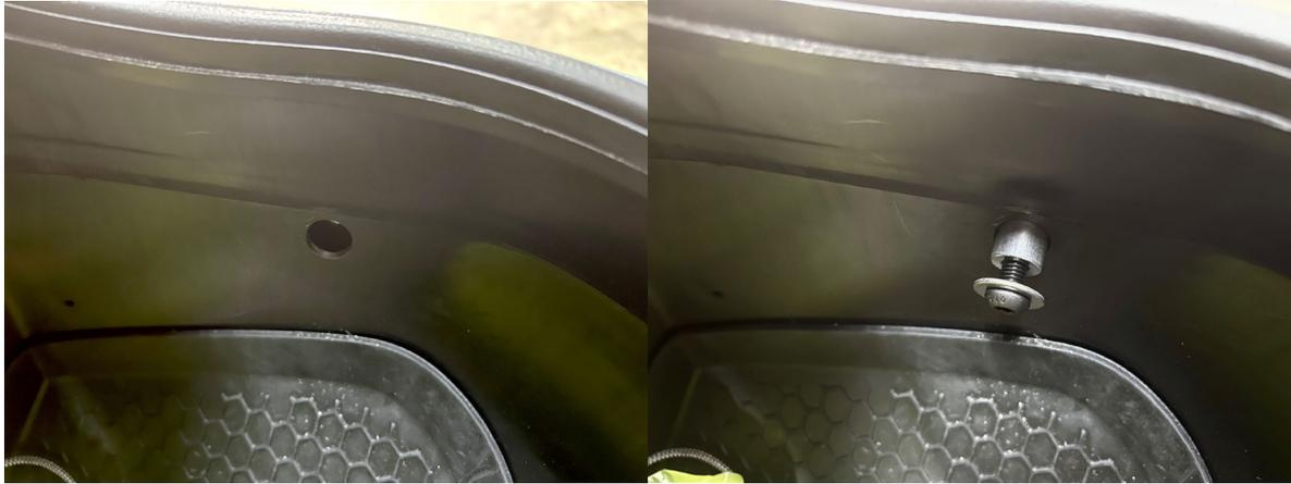
3.-Locate the bolt washer and spacer. Take the washer, place it on the bolt then add the spacer. Place through the hole as shown above then apply the flag holder to the outer trunk side once the paper template is removed.
