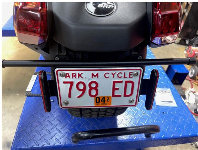
4.- Once installed you can take the flag, remove the two socket had bolts from the bottom of the mount and then place the flag on the mount shaft as shown below. Slide the flag over to the rubber end cap. Tighten down after you have located the flag at the angle you like best. Tighten down and your flag and your flag kit is installed!
