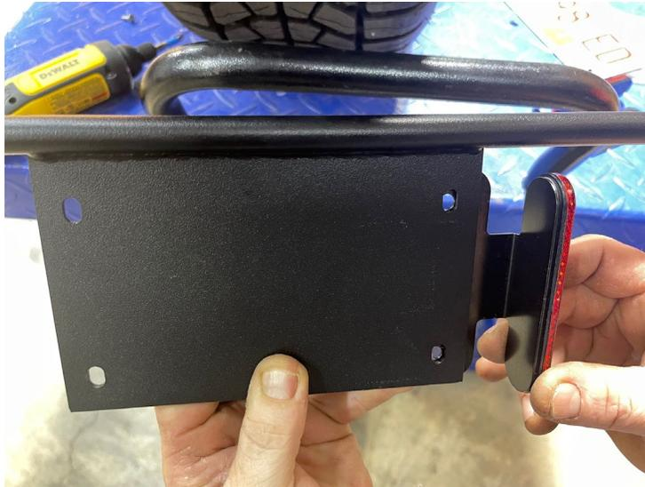
3.- Then take the license plate while holding each reflector and use the four supplied bolts and screw them to the flag mount left & right brackets using the bolts holes in the center of each bracket.
