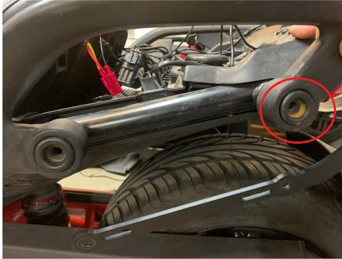
3.- When adding the new rear trunk rack assembly, it is best to have another person to help hold the mount in place while adding the spacers and bolts below. **Start with the rear bolts Circled in Red above both sides first. Do one bolt each side at a time.**
