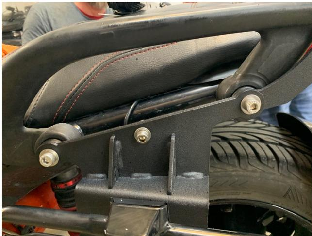
5.-Install the rear mount first then add the saddle bag brackets on top of the rear trunk mount as shown above.
