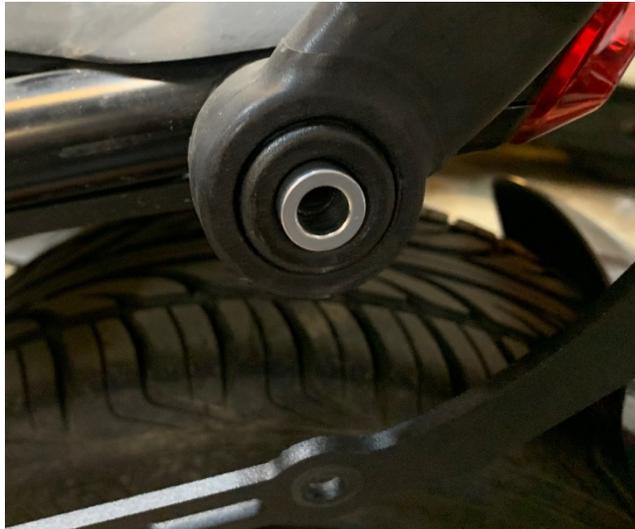
4.- Install the aluminum spacers as shown above in each location.
