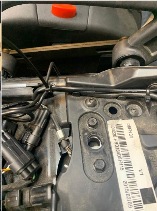
7.- Now check all wiring to assure that the brake, blinker and driving lights are working. If so, install the rear passenger seat and lock the rear trunk in place. Make sure, again the left & right taillight wires for the trunk are plugged in and working.
