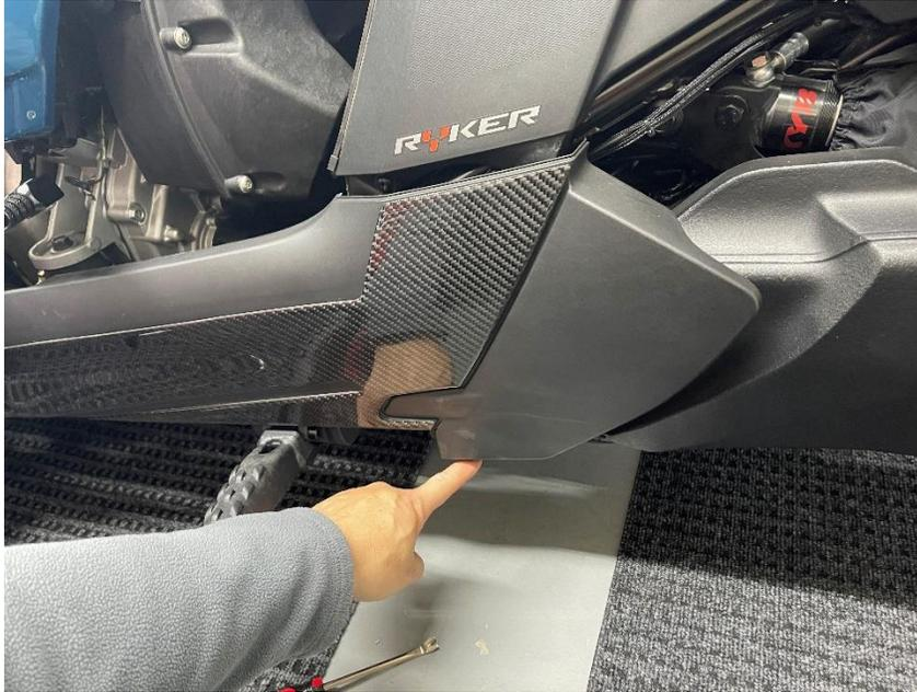
5. Locate the final push pin on the bottom of the side fairing in the rear to remove it.
