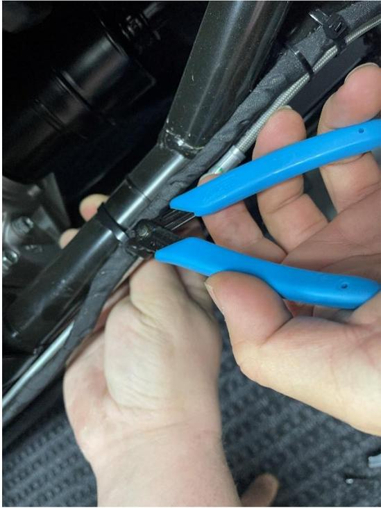
9. Cut the zip tie on the horizontal frame rail close to the rear where it y's off.
