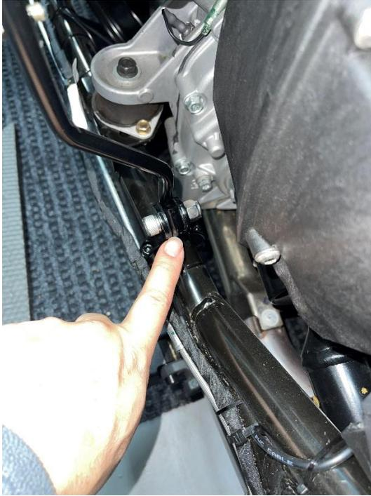
24. Come back through making sure all bolts are tight including the frame brackets which were loose up to this point.
