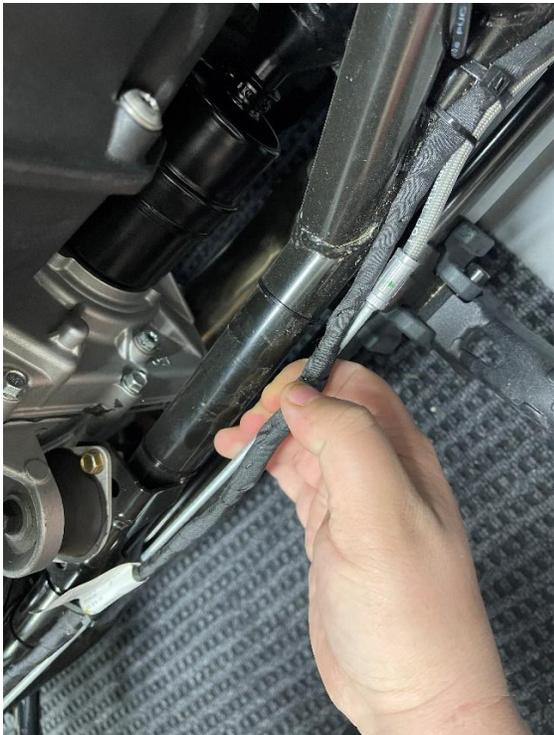
10. Gently pull back on the wiring and brake line to make sure there will be room to slide your frame mount bracket.
