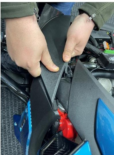
1. With the front hood removed pull down and towards the front of the bike on the front nose fascia to slide it off.
