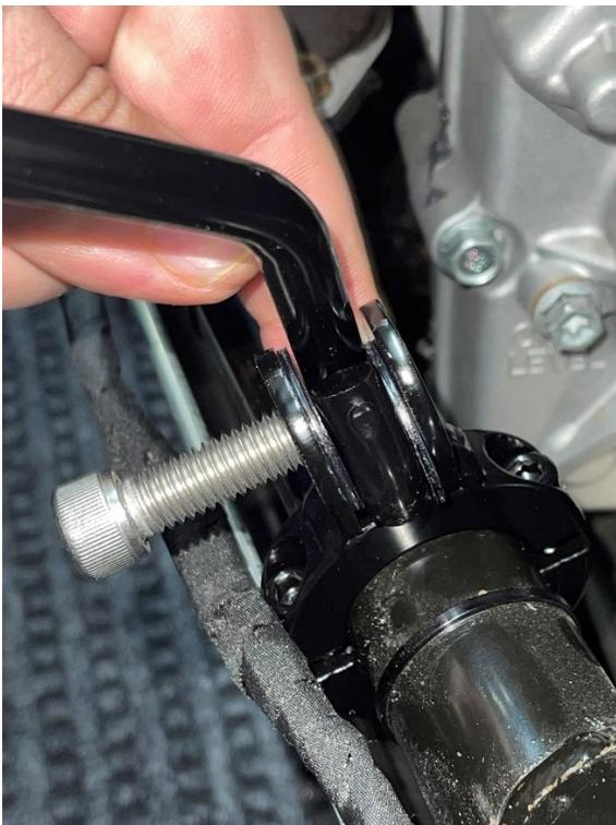
16. Place the vertical shaft in the middle of the two nylon washers and push the bolt through.
