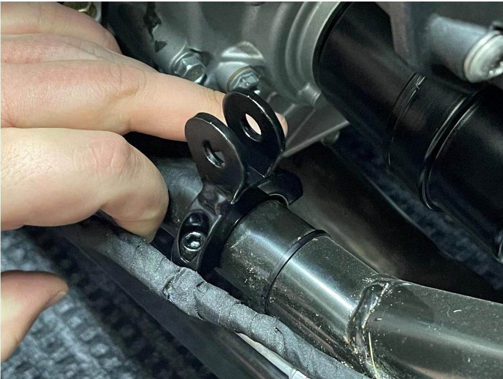
12. Lightly pull back the brake line as well as the wiring to affix the frame mount brackets.
