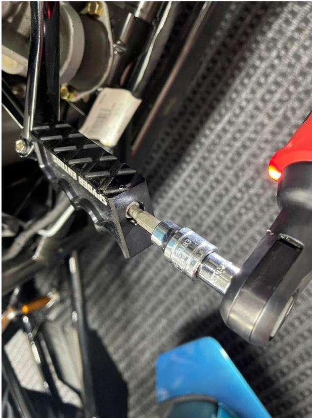
8. Remove the factory torx 30 bolt from the side of you gear shifter.
