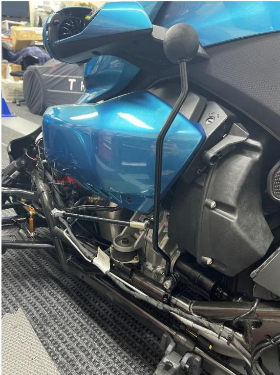
25. Screw your gear shift knob on the stop of your hand shifter and then re attach all panels going in the reverse of removal.
