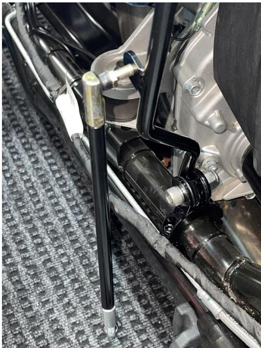
19. Push the end link bolt from the horizontal shaft through the bracket on the vertical shaft as shown.
