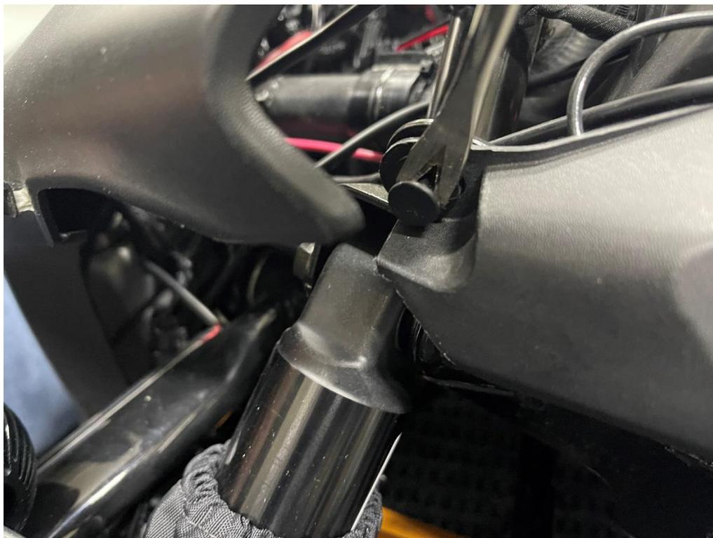
2. Remove the push pin revealed by step 1.
