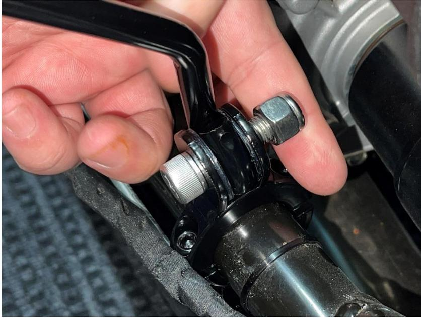
17. Attach the locking nut to the back and tighten until it is somewhat snug. Do not fully tighten yet.
