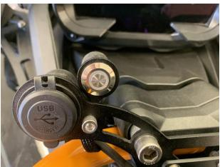
2.- The wring is simple. The Black wire is ground, The Red wire is the power source and the White wire is the output to your device to be switched. There are many uses for the switch from LED Driving lights to Audio Accessories.
