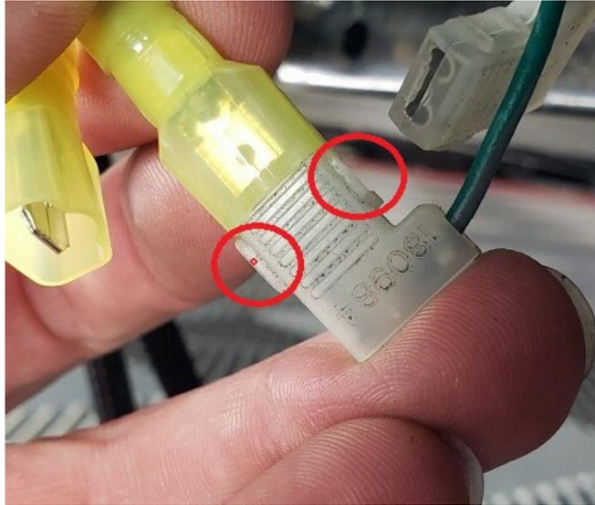
Then connect the pairs of horn wires to each horn. Again, it makes no difference which connector for each horn is on what terminal. No polarity to deal with. They are grouped in pairs, so each pair connects to each horn. Tie the new harness to the frame area with the new wire ties.
