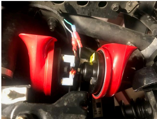
8.- Take the wiring harness and connect the ground terminal next the relay to the ground post on the battery and connect the red fused wire to the positive battery terminal. Take a wire tie and secure the relay to the left of the battery negative wire secured to the factory harness.
