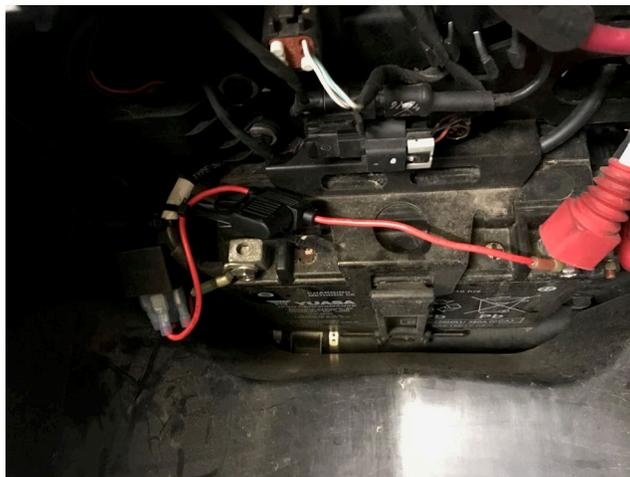
9.- If you look to the left of the battery, you can see a space to run that harness to the horn location. Once at the horns, remove the terminals of the existing horn wire. You will see the new harness as two wires with butt connectors. Those are the wires that trigger the new horn relay from your existing switch. Take those existing switch wires and connect them to the existing horn switch wires. It makes no difference which wire goes to what butt connector.
