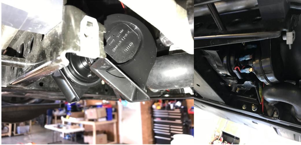
**6.- Got back to the battery location and connect the red power wire to the battery. Then test your horns. Beware that when these horns blast the sound is much louder than the factory. If all works, take the wires ties and tie up any loose ends of wires and then reinstall the lower plastic cover. Then zip backup the trunk liner and your horns are installed**
