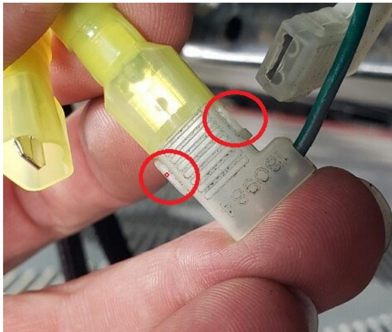
Make sure the center spade on the yellow connectors is straight in the yellow housing to allow it to connect to the existing horn plugs. The existing horn wire now controls the relay only that powers the new horns. Then take the pair of red/black horn wires and plug them in to each or making sure negative is negative and positive is on positive.
