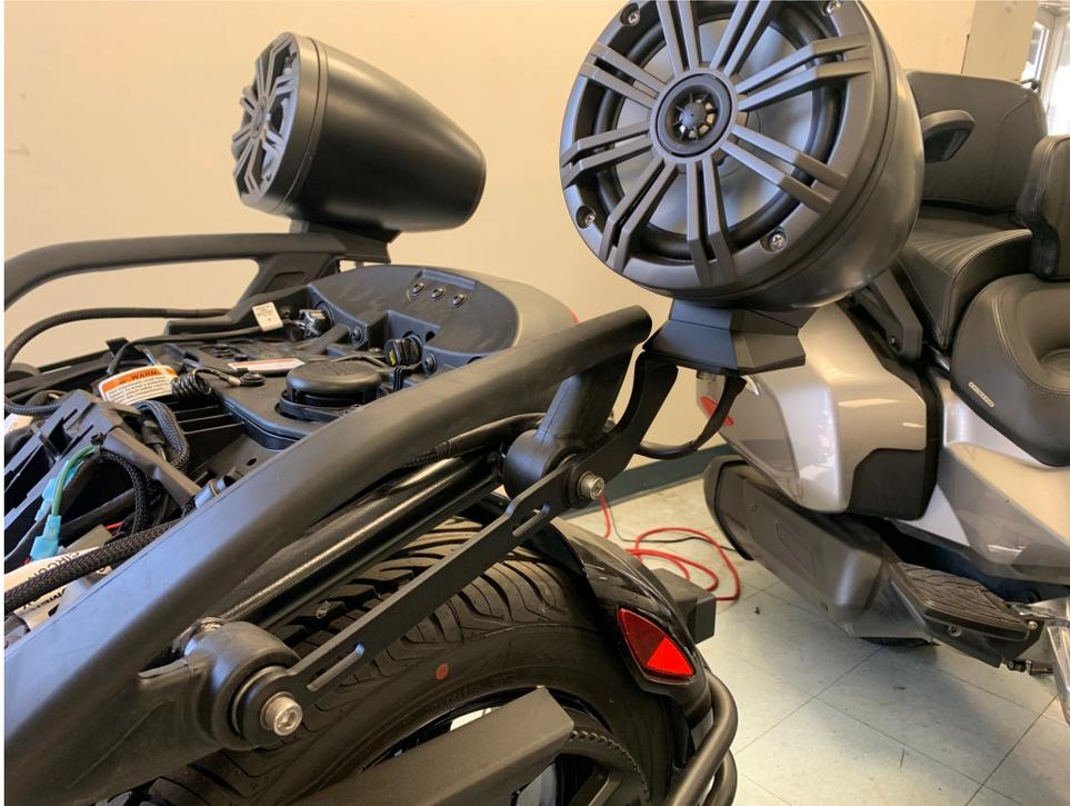
10.- Once all speakers are installed and secured to your Spyder Turn on Switch #1 on the left on your docking station to test your system. At this point all should be installed, amp in the trunk secured with all wires connected including the power and ground wires to the battery, satellite radio model installed and both antennas.
