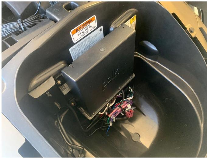
5.- This kit comes complete with the FM Antenna and a Satellite Radio Module that plugs into the back of the amp unit. The Polk Head unit on the Docking station will know when the module is plugged in. Like any Satellite Radio you will need to have a Subscription.
